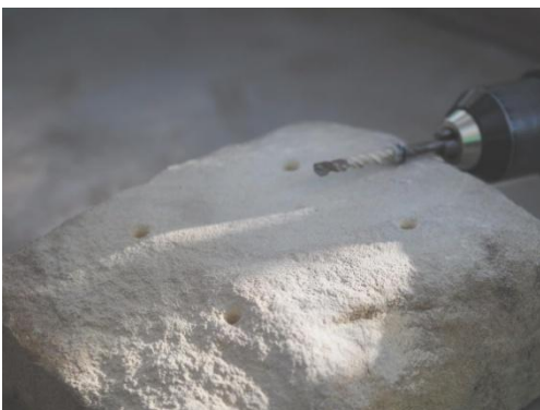
3.) 4 x holes drilled to a depth of 45 mm – I use a bit of bonsai wire on the drill bit as a depth indicator.
