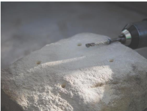
3.) 4 x holes drilled to a depth of 45 mm – I use a bit of bonsai wire on the drill bit as a depth indicator.
